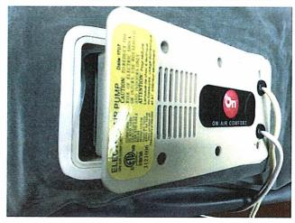
Step 5: Must ensure the gasket is sitting flat in the designate groove in the frame before the replacement motor is installed. The gasket may adhere to the pump motor that was removed. If it does, carefully remove the gasket and then properly place and position in the frame. Do not use a sharp object as this may damage the gasket. Do <u>not</u> glue the gasket into place. (Note: The blue paper is <u>only</u> used to make the gasket more visible for instruction and picture purposes.)
