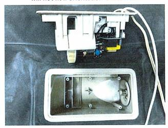
Step 7: Using a phillips head screwdriver, install the six (6) screws by turning clockwise. Do <u>not</u> overtighten the screws. The screws should be finger-tight (i.e., snug) plus ¾ additional turn. This will avoid stripping the screw thread in the mounting frame.
